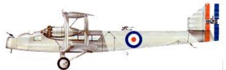
A wooden airframe Handley Page Hyderabad from which the all metal airframe Clive airliner was derived.
